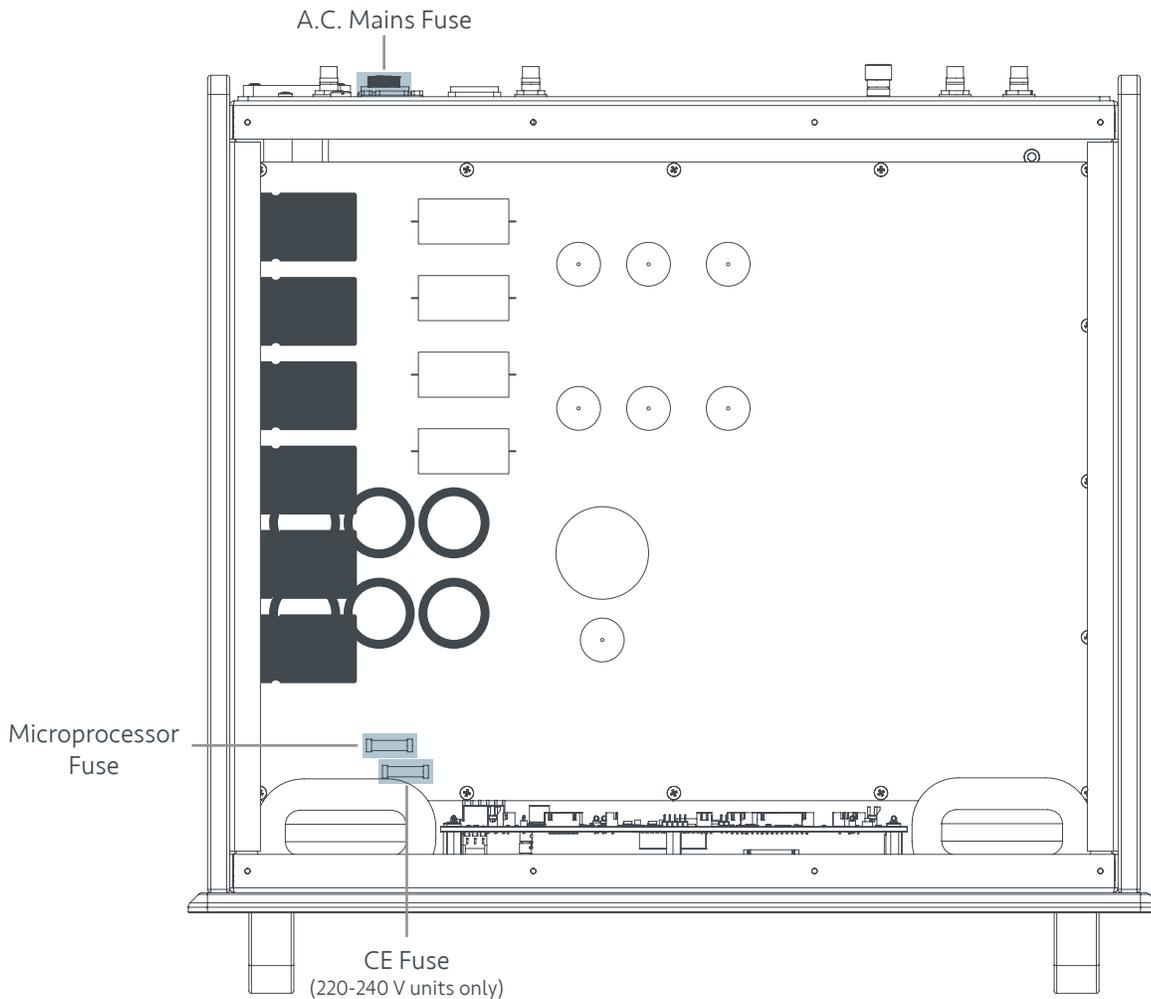
The Reference Phono 3 has three replaceable fuses to help protect the unit in the event of a spurious electrical surge or other situation. When replacing a fuse, please use only the specified rating and type. Using an improper rating or type, or bypassing the fuse, will not only void the warranty in the event of damage, but it could also cause serious system failure, fire, or personal injury.
