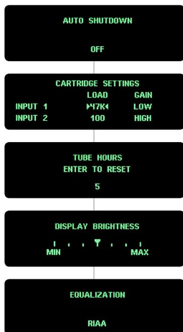
While a menu item is displayed, press 'OPTION' on the front panel or remote to adjust the settings of that particular selection. After making the appropriate change, pressing the 'ENTER' button will confirm the new setting, and the display will show 'OKAY' for five seconds before reverting back to the normal operation screen.
