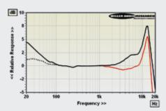
ABOVE: Frequency response curves (-8dB re. 5cm/ sec) lateral (L+R, black, Output 1; dashed, Output 2) versus vertical (L-R, red Output 1)
