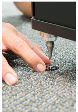
8. Once positioned, adjust the thread depth of the spikes so that the speaker is level and all four spikes are firmly coupled to the floor without any wobbling of the speaker. Tighten the nut on the spike upwards firmly to the bottom of the threaded puck to secure the spike in place.
