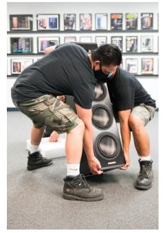
6. While one person tips the speaker back, apply the spikes to the threaded pucks on the front of the speaker. Tip forward and repeat for the rear spikes.
